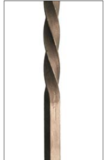
Mill scale on twist baluster
