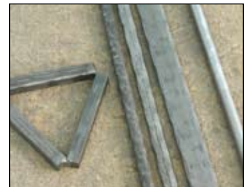
Hot rolled steel with one cold rolled round bar
